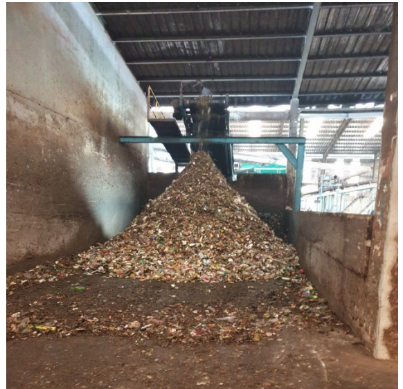
Figure 14 Organic waste at the end of the sorting line (Source: Hoai Le, evaluation team)
